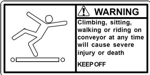
#111752 (5" X 2 1/2" ) Placed on max. of 20' centers (both sides) along conveyors which provide surfaces and profiles attractive, but hazardous, for climbing, sitting, walking or riding.
