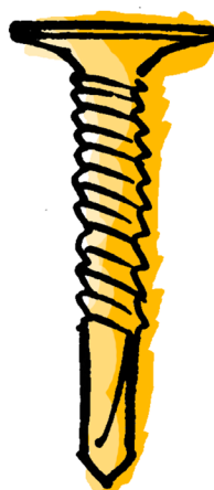
\varnothing 1/4'' \times 1'' FLAT HEAD TEK SCREW
